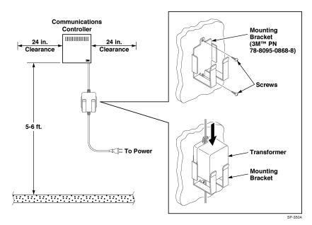
Figure 2. Suggested Communications Controller Placement
